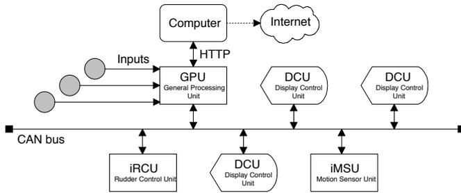
Figure 3. RoboSail's CAN-based network architecture
